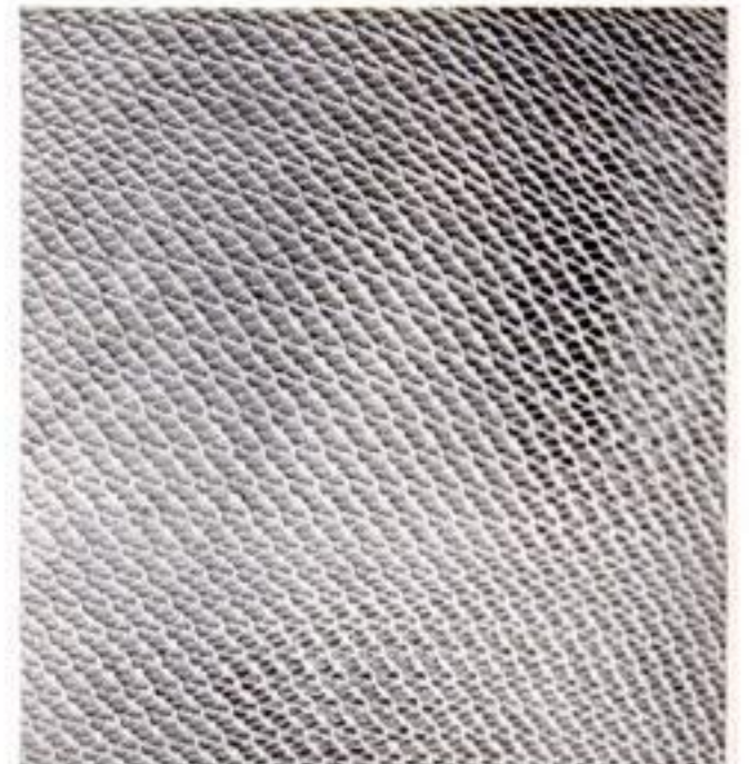
Eyelet batiste plus Lastex mesh is used for the all-in-one. Its weight: 2 5/8 oz.
